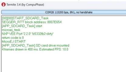
→ This board is theoretically able to run GUI applications near 60FPS. The next steps are about investigating the bottlenecks in the application and in the VEE Port that prevent having a smooth animation.
